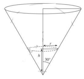
Let r be radius, h be the height,  $\theta$  be the semi-vertical angle and V be the volume of the water at any time t.
